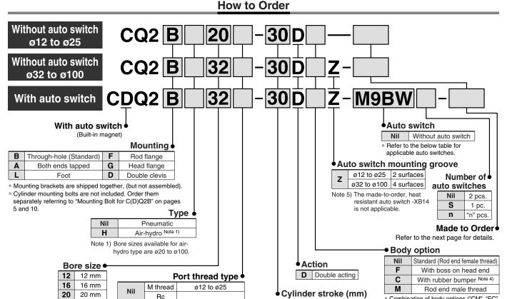
Built-in one-touch fittings Note 2) Note 2) Bore sizes available with one-touch fittings are Ø32 to Ø63. Besides, it is not possible to use for air-hydro type.
